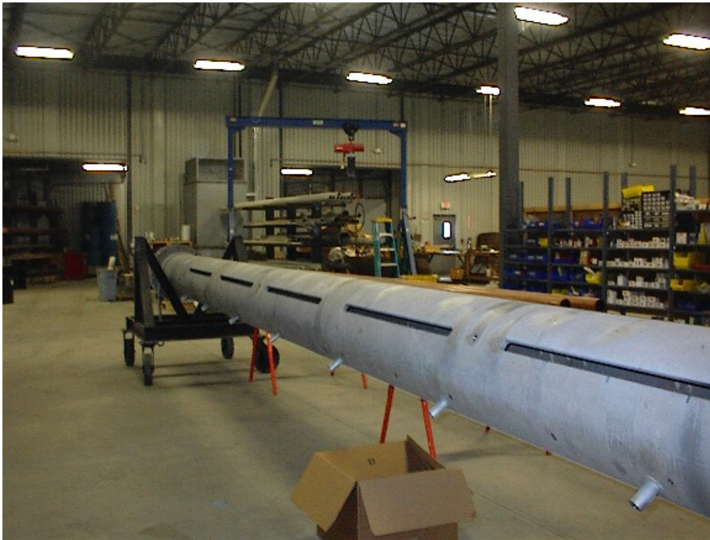
A 3 slot around Omni-directional VHF Pylon antenna on channel 13
